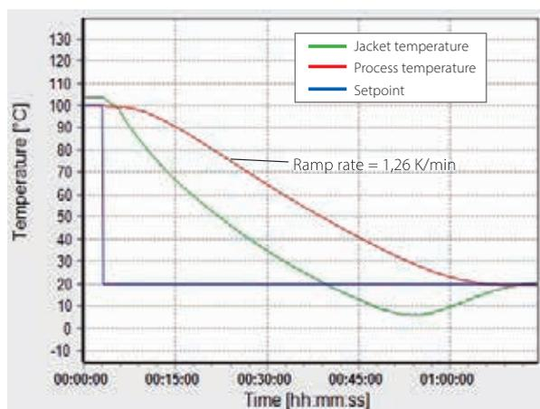
The second graphic shows the time taken to cool the process from 100°C to 20°C. It can be seen that the time taken is approximately 64 minutes, again the stability and accuracy of the control is clearly demonstrated.
